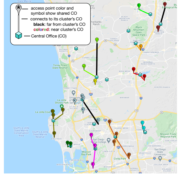
Figure 16: Inferred EdgeCOs for access points (APs) in a San Diego ISP. Marker color identifies APs connected to the same EdgeCO. Black lines indicate that the EdgeCO is not the closest CO.
